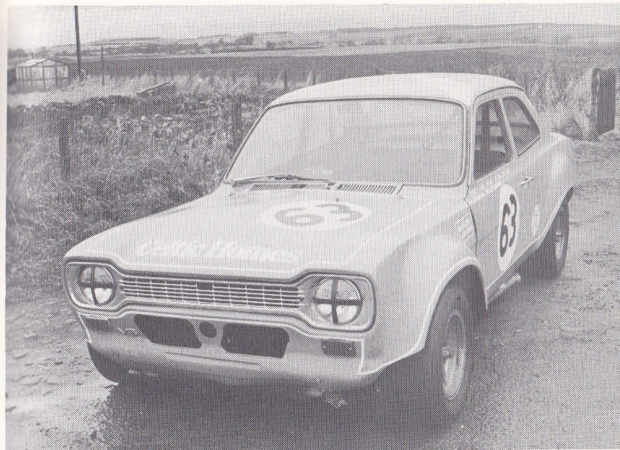
The Celtic Homes Boss Escort, above, showing the extra wide racing slicks on March F1 wheels. The tiny V8 symbol on the front valance (left) gives the secret away. The motor (Below) is 5.7 litre Ford Boss Mustang with Mathwell heads mounted tight up against the bulkhead and cooled by twin radiators with the oil cooler between.
